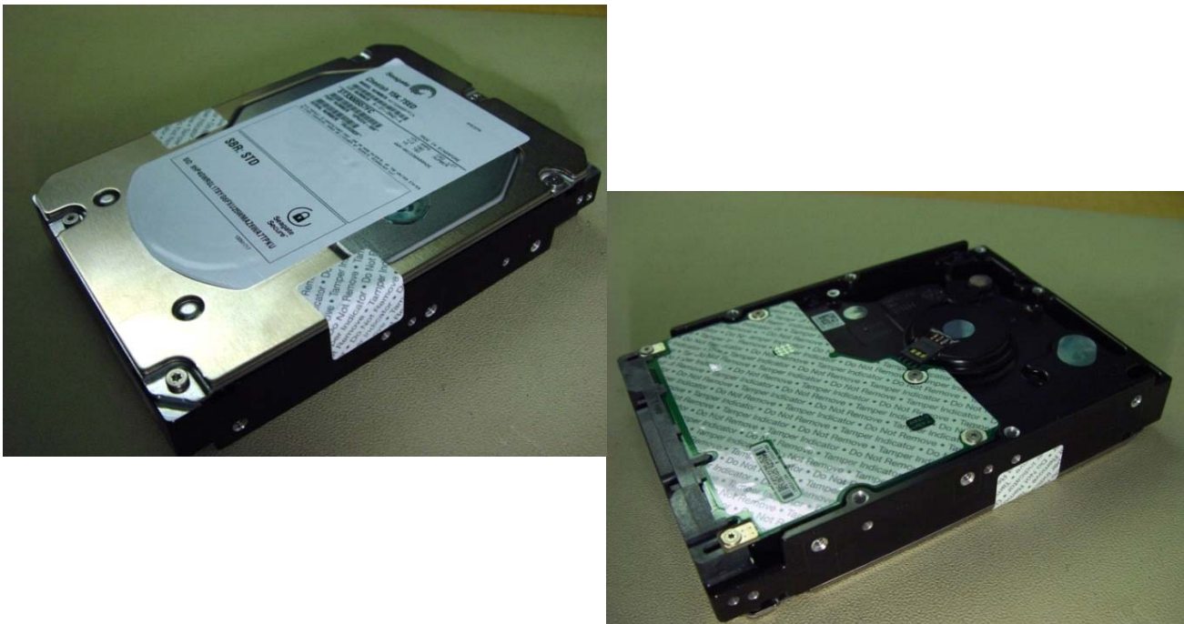
Figure 7. Example of FIPS tamper evidence labels.
