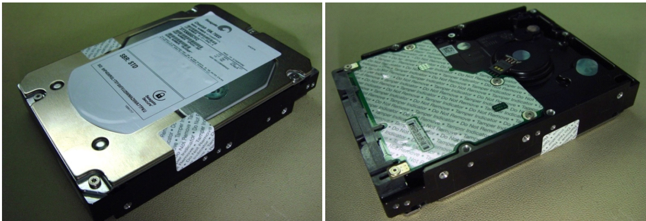
Figure 8. Example of FIPS tamper evidence labels.
