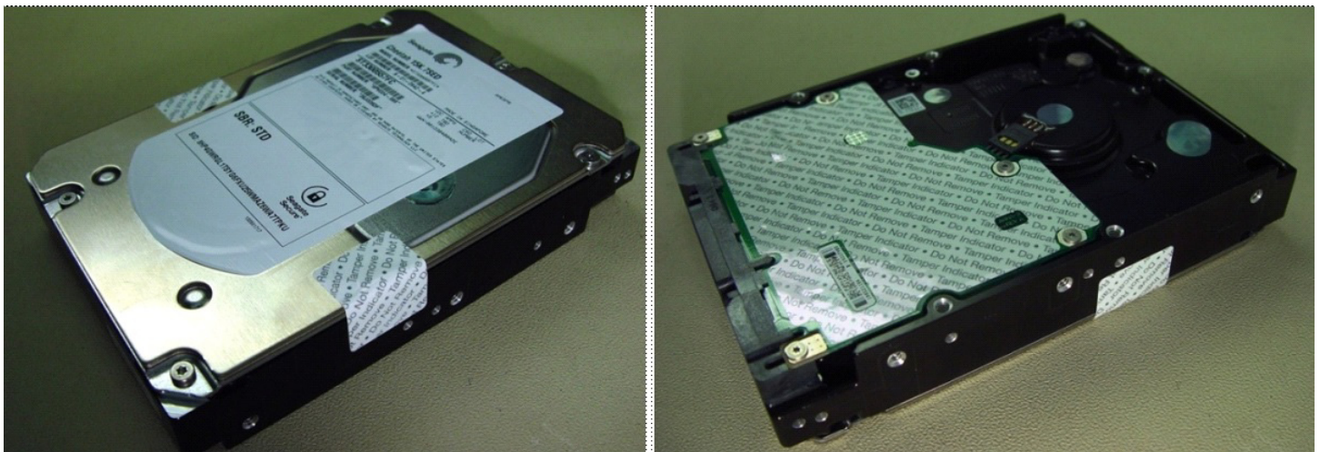
Figure 5. Example of FIPS tamper evidence labels.
