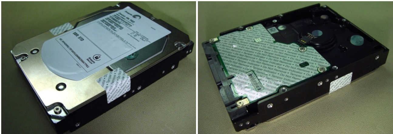
Figure 12. Example of FIPS tamper evidence labels/seals.
