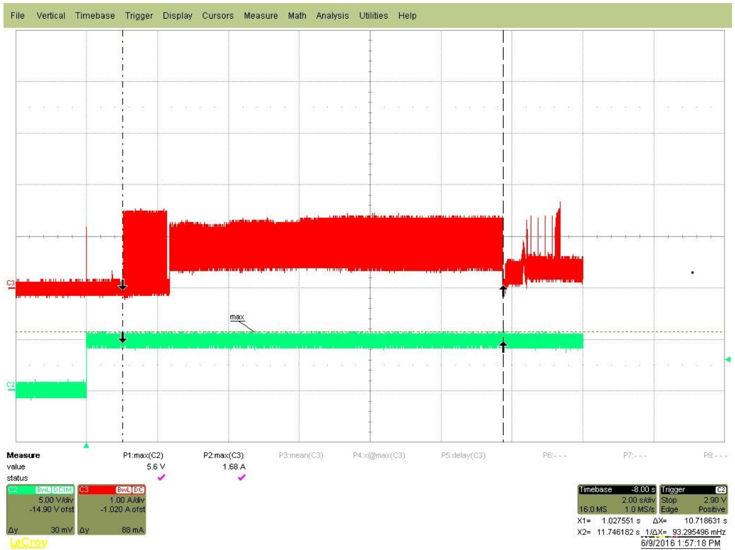
Figure 1. Typical 5V and 12V startup and operation current profiles (10TB & 8TB)
